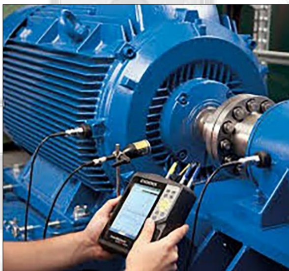
Figure 1. Vibration measurement of the motor
