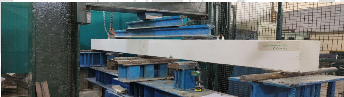
A) preparation of the specimen for testing
