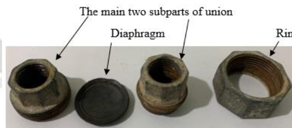
Figure 1 Real union fitting parts with the diaphragm
