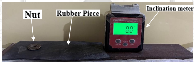
Figure 21 Experiment details to compute the coefficient of Friction
