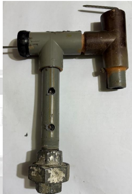
Figure 37B Real improvised Pressure Switch
