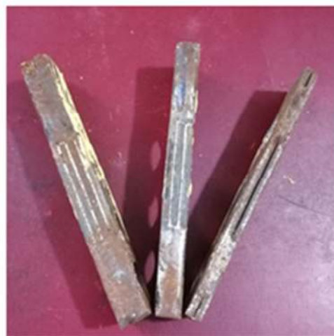
Figure 1 –B Blades dimension 100 mm Length x 25.4 mm width with different of thickness 6 , 9 and 12 mm
