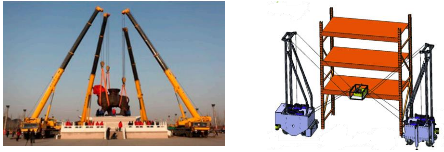
FIG. 4. (LEFT) A COOPERATIVE CRANE SYSTEM BEING USED TO MOVE AN HEAVY OBJECT [18]. (RIGHT) A CDPR MOUNTED ON TWO MOBILE PLATFORMS [19].
