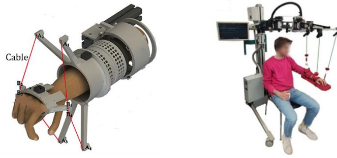
FIG. 5. (LEFT) EXSKELITON CDPR FOR HAND REHABILITATION [31]. (RIGHT) END-EFFECTOR CDPR FOR ARM REHABILITATION [32].
