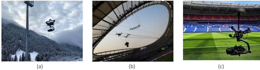
FIG. 3. (A) 1T CABLE CAMERA SYSTEM (B) 2T CABLE CAMERA SYSTEM (C) 3T CABLE CAMERA SYSTEM.
