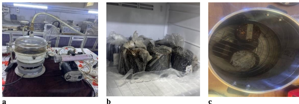
Figure 8. Tensile Strength Ratio test Procedure (a)Vacuum process , (b) Freezing of specimen, (c) water bath @ 60^\circ\text{C} for 24 h.
