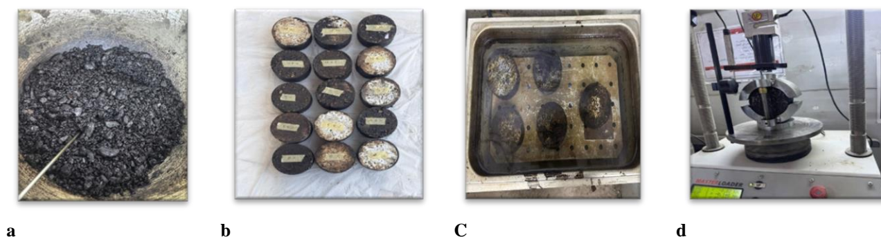
Figure 5. Marshall test procedure (a) Preparing mixture, (b) Group of Samples, (c) Water Bath, (d) Test Running
