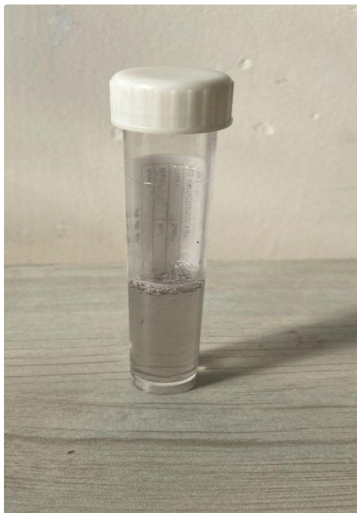
Fig (1) Nanoparticle synthesis by pulse laser ablation.
