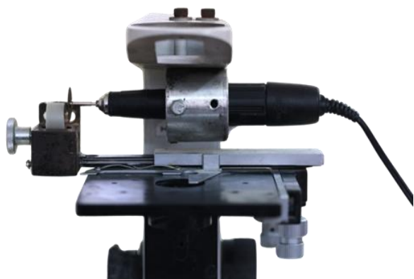
Figure (1): flattened labial surface using locally modified microscope
