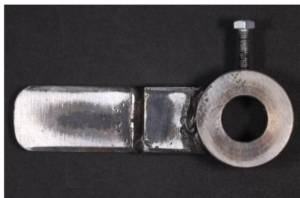
Figure (4): Locally made metal holder used for universal testing machined device for shear bond strength test.
