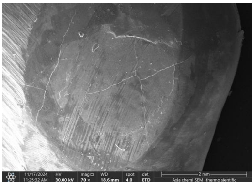
Figure 6: The representative SEM image at 70X magnification shows an adhesive fracture.
