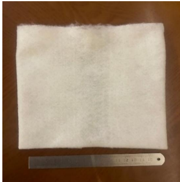
Figure 3: Nonwoven geotextile (PET NW130)
