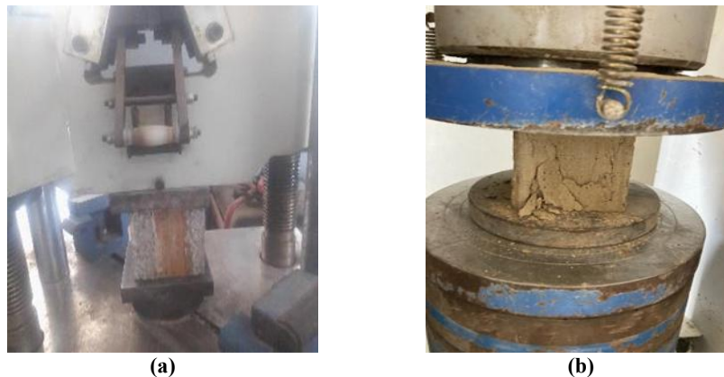
Figure 3: a) Compressive strength test, b) Failed sample at compressive strength test
