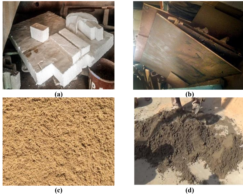
Figure 1: a) Samples of expanded polystyrene, b) Samples of particle board, c) Sand aggregate, and d) Cement mortar mixtu
