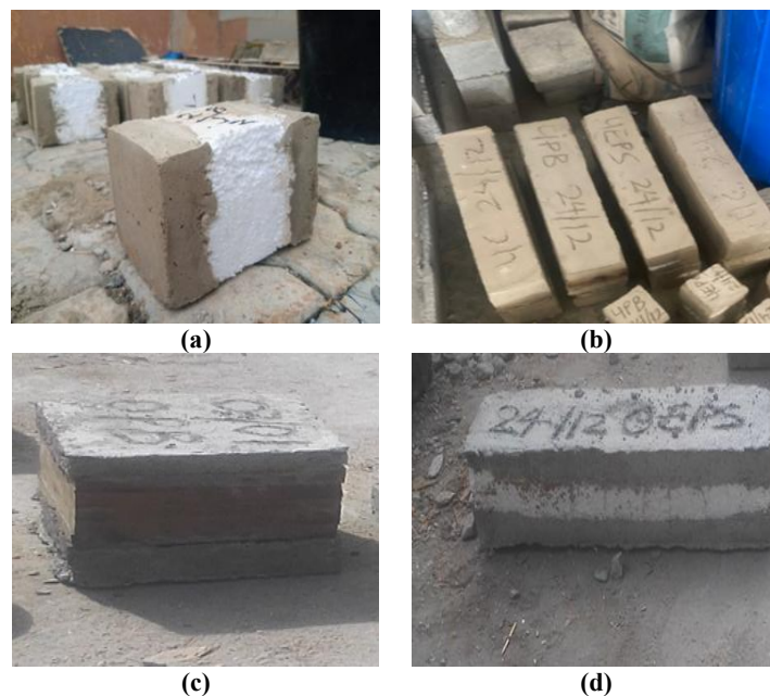
Figure 2: a) Samples of EPS core, b) Samples of PB core sandwich Sandwich Panel, c) Sample of EPS core Sandwich Panel d) Sample of PB core sandwich panel
