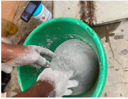
Figure 3: Manual dry mixing of sawdust, cement, and calcium carbonate
