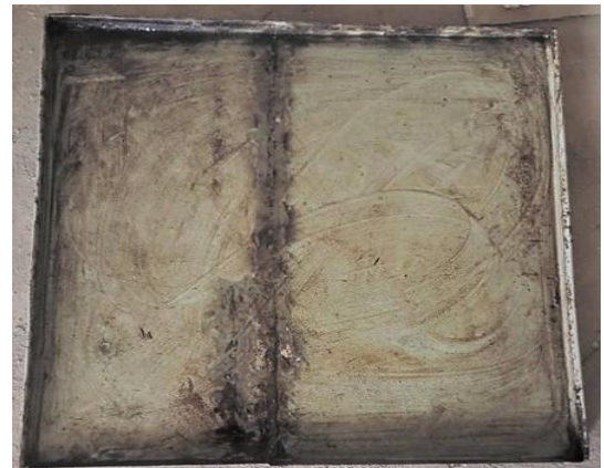
Figure 2: Custom-fabricated mild steel mold used for shaping sawdust-cement composite ceiling boards
