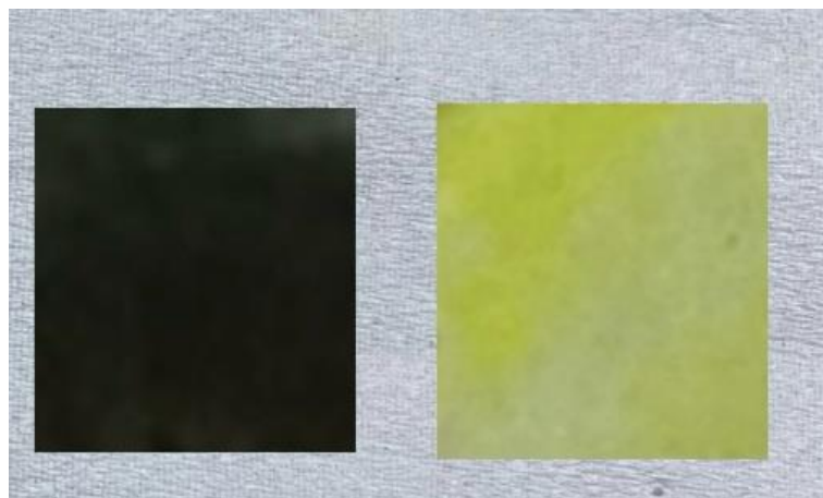
Figure 6: The MAPI visual sensor's reaction to a change in color.
