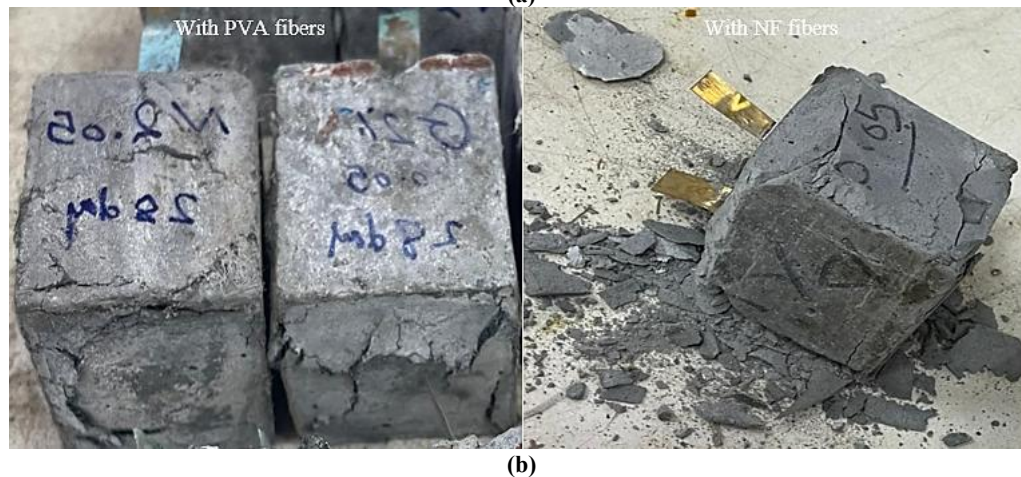
Figure 3: a) compressive strength for various innovative blends during curing age, and b) Samples after testing
