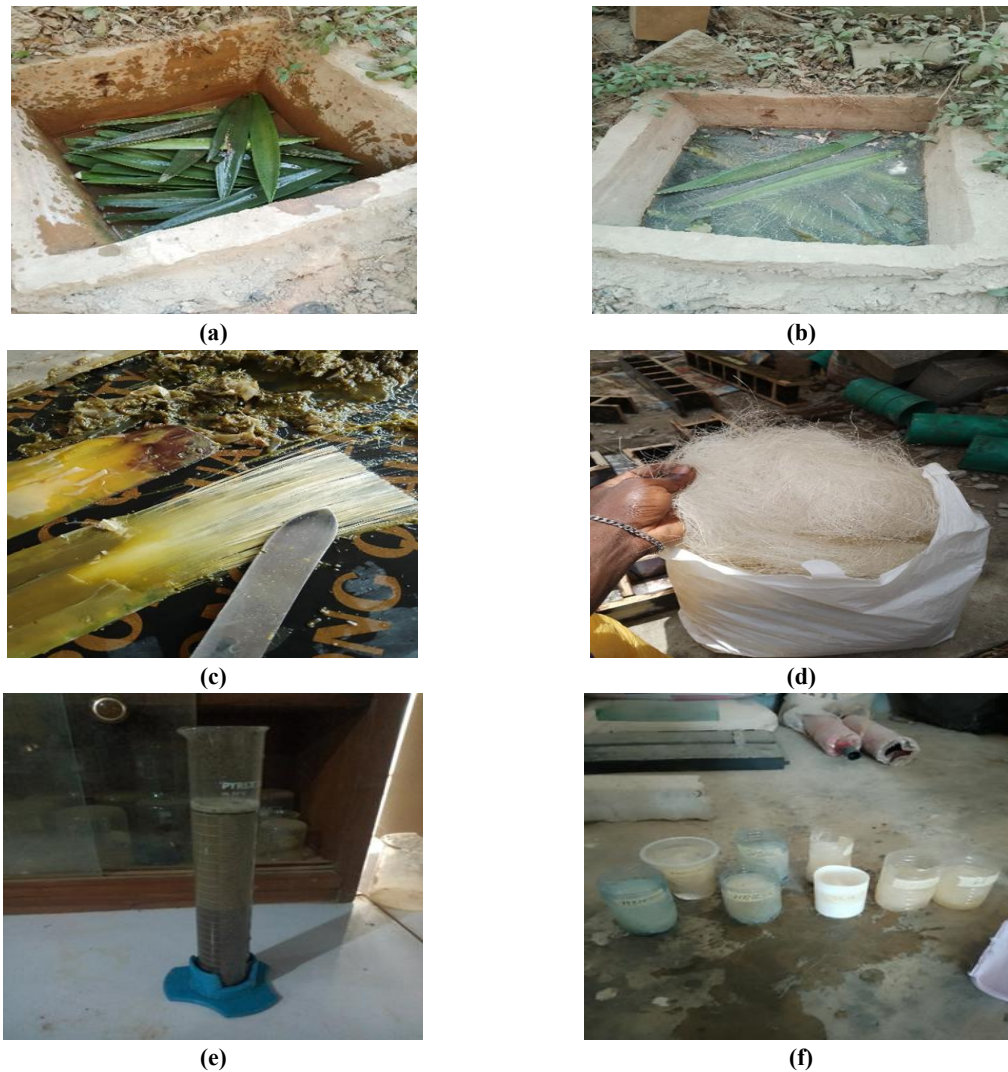
Figure 2: a) Cleaning of henequen leaves, b) Soaking of henequen leaves, c) Decortication process, d) Extracted henequen fiber, e) Solution of sand sample for Silt content determination, f) Water absorption test on fibers
