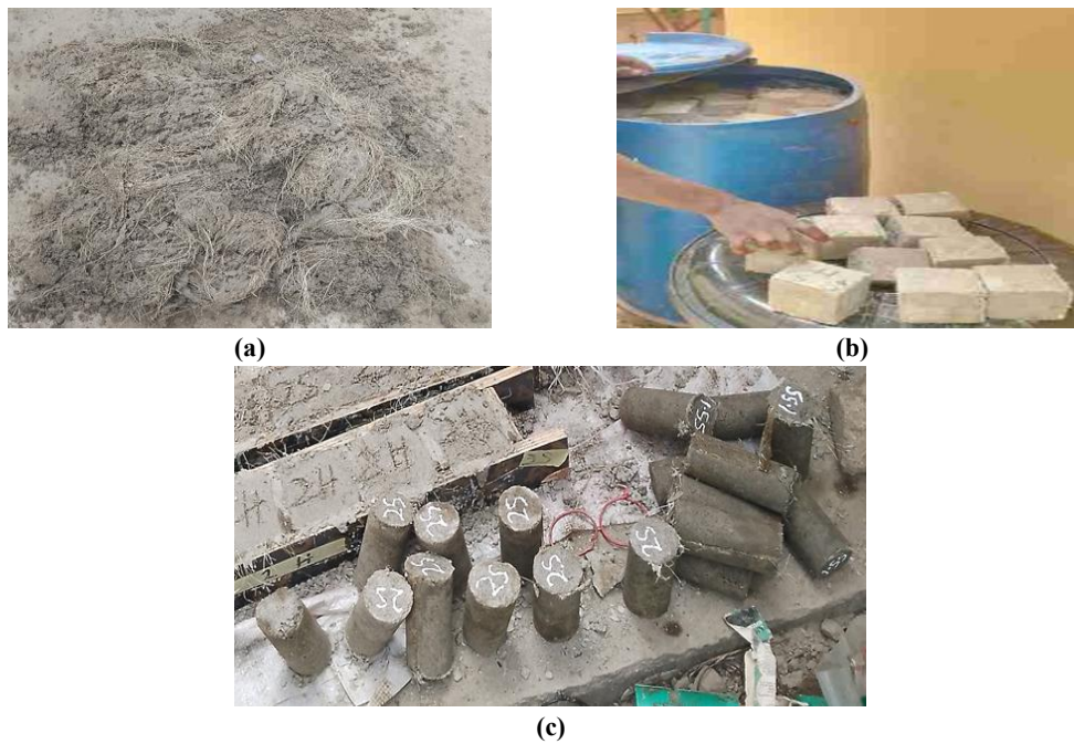
Figure 3: a) Fiber incorporated into fresh mortar sample, b) Cube mortar samples, c) Cylinders mortar samples
