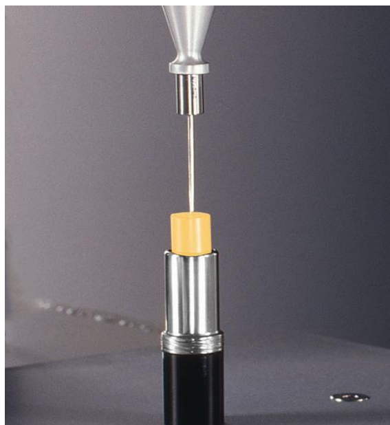
Figure 6 illustrate thixotropy test.
