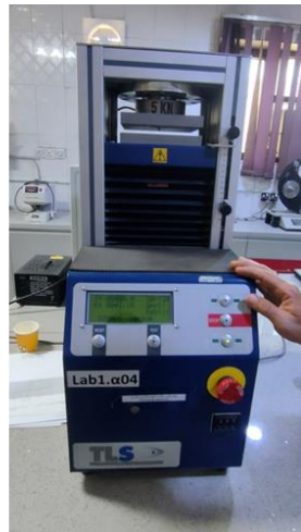
Figure-2 the Techlab Systems Instron Universal Testing Machine
