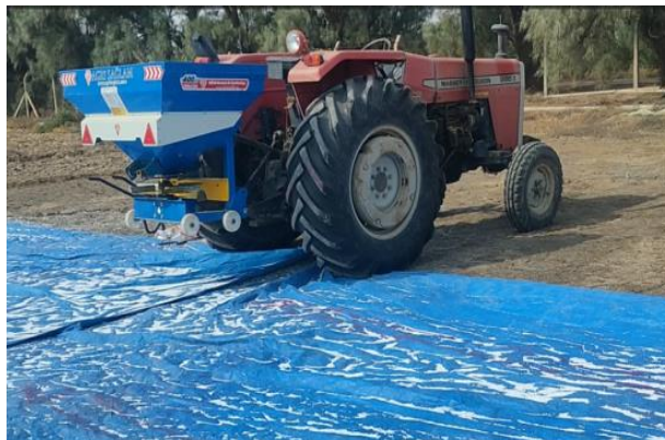
Figure–1 Agri Saglam 400-liter single-disc fertilizer spreader Connected with Massey Ferguson 285S tractor
