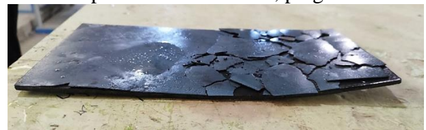
Figure 5. Peeling surface layers and deformation (bending) of large specimen
