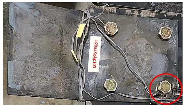
Figure 3. Location of strain gage on specimen
