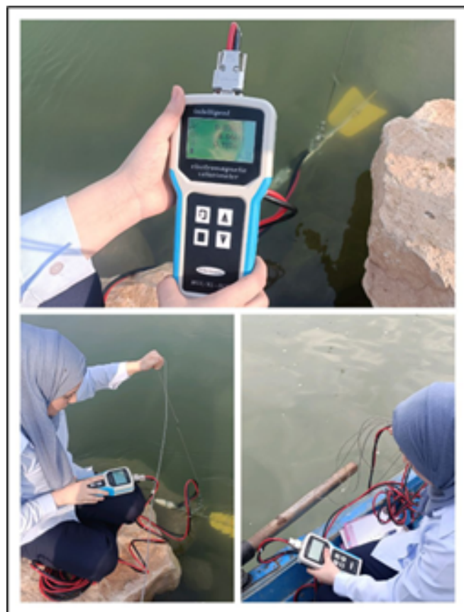
Fig. 2 Current velocity measurements from a boat
