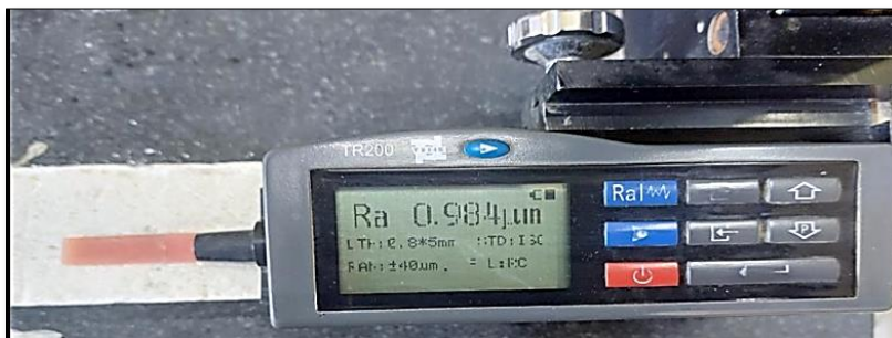
Fig. 2. Specimen is subjected to surface roughness test
