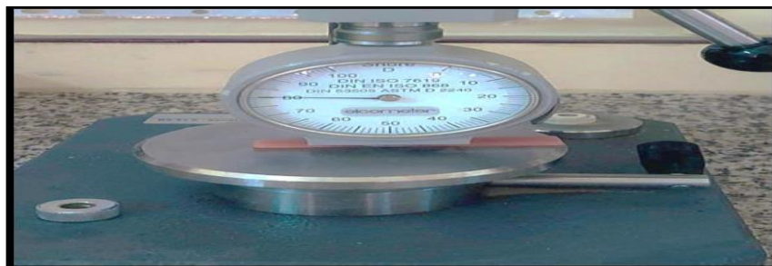
Fig. 3. Shore D dourmeter tester device for measuring the surface hardness of the heat acrylic resin specimen
