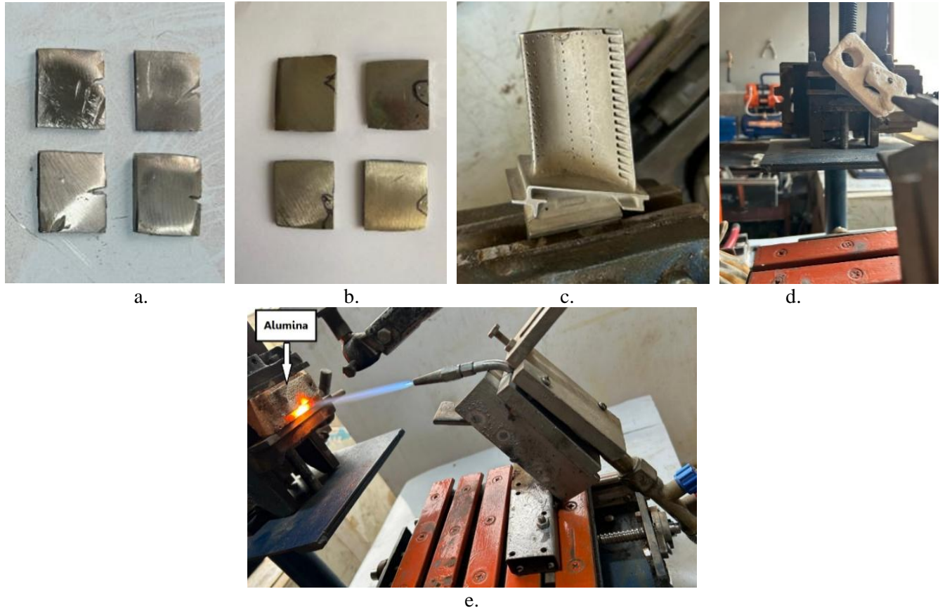
Figure 6: a) samples before repair, b) samples after repair, c) HPTB after repair, d) protective shield Alumina, e) using the FTTHS technique for repair.
