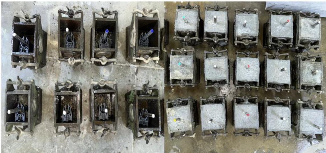
Figure 1. Cubic concrete specimens before and after casting.
