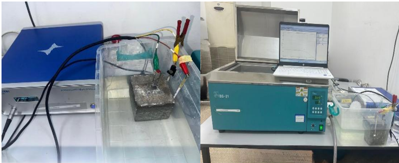
Figure 2. Electrochemical measurements using a three-electrode cell.
