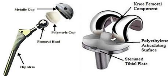
Figure 3. Schematic diagram of artificial hip joint (left) and knee implant
