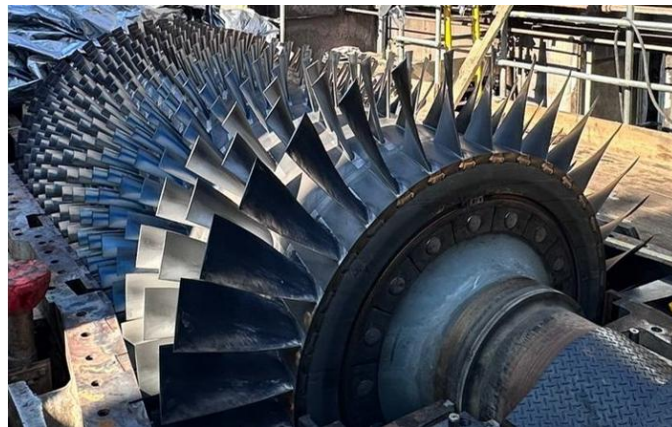
Figure 6: Compressor blades of frame 9 from the GE company
