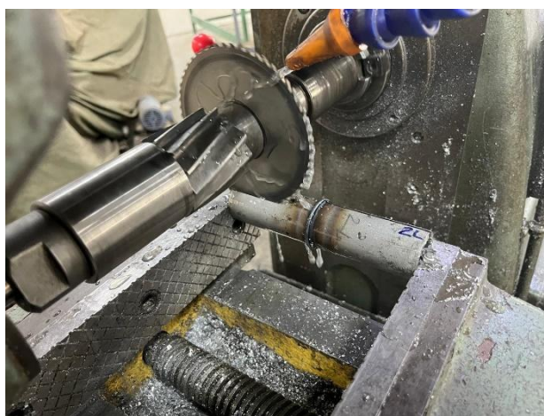
Figure 3: Cutting process for the welded pipes during sample preparation
