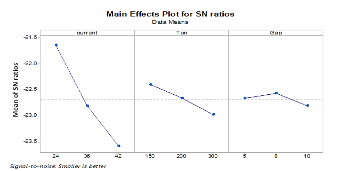
Figure 13: The S/N main effects plot for the SR
