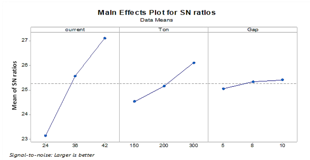
Figure 12: The S/N main effects plot for the MRR
