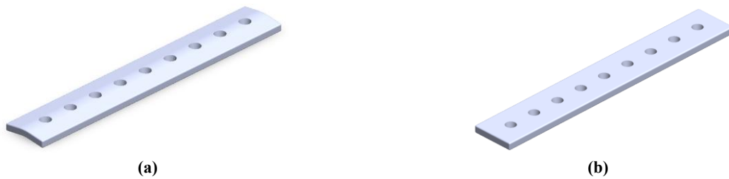
Figure 2: Showing an isometric view of a locked bone plate: a) Traditional Flat Plate, and b) bent plate
