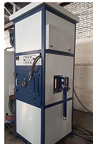
Figure 2: a) Diagram of the RF sputtering process [24], and b) RF sputtering system
