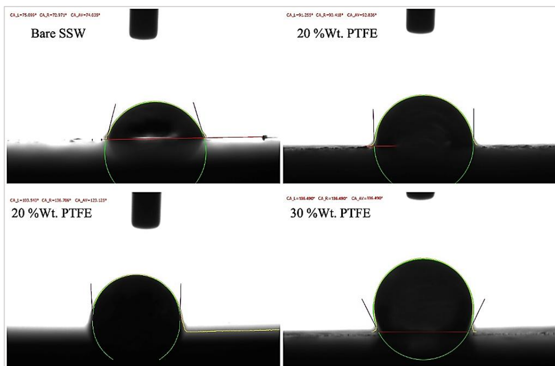
Figure 10: Contact angle measurements for the uncoated SSW and Ag-PTFE coated SSW at different weight percentages of PTFE
