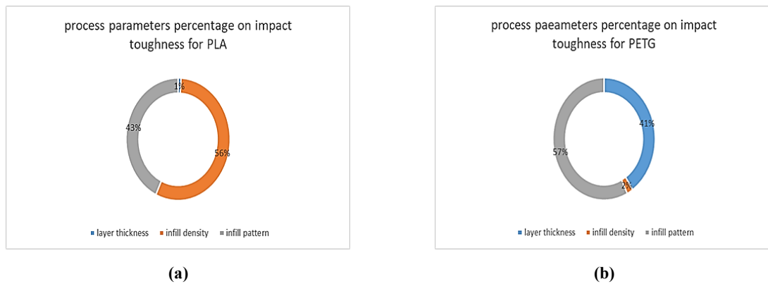
Figure 2: Percentage printing parameters on impact toughness for a) PLA, and b) PETG
