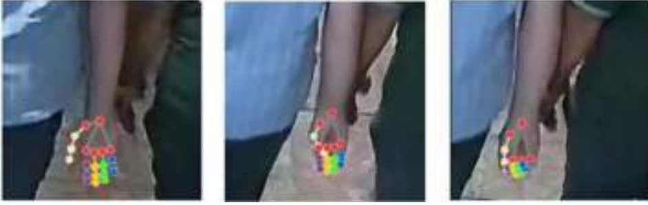
Fig. 4. Illustrates the tracked hand after using the MediaPipe Hands framework similar to the Body pose illustration. As shown in the above figure, this process involved.
