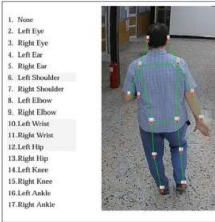
Fig. 3. Keypoints that extracted through the implementation of YOLOv8n pose estimation.
