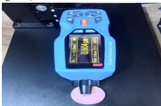
Figure 4: A profilometer was used to analyse the roughness of the diamond surface analyser.
