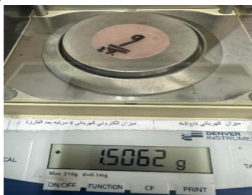
Figure 6: Measurement of specimen mass using an electronic balance with an accuracy of (0.0001\text{ g}) .
