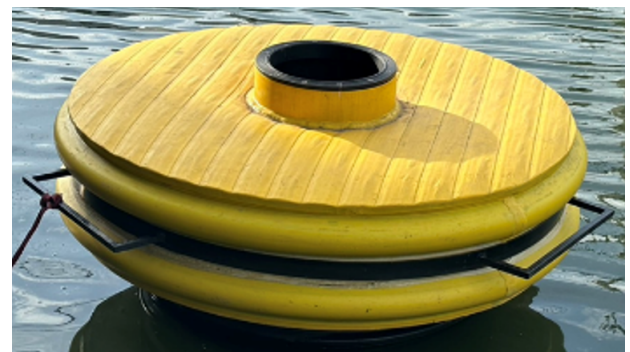
Figure 7. General appearance of the smart pontoon fabricated with colored reinforced HDPE during its test.
