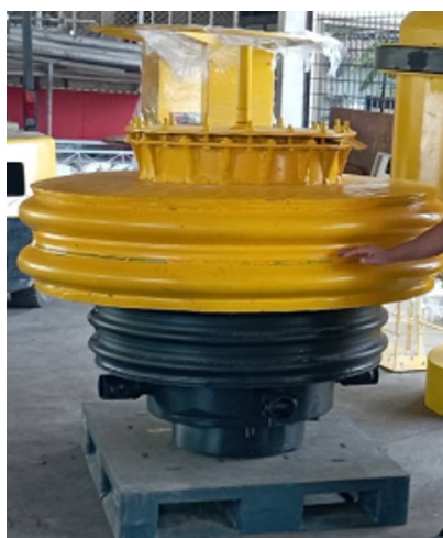
Figure 6. Physical appearance of the smart pontoon fabricated with colored reinforced HDPE.
