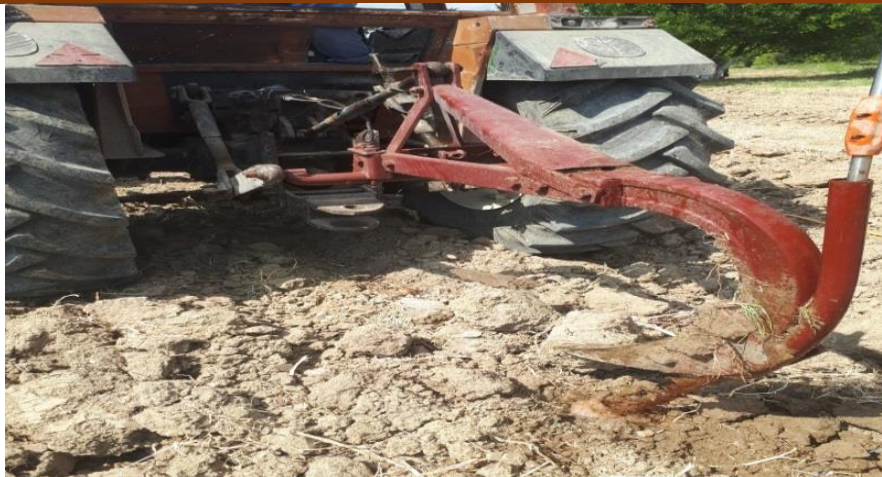
Figure 1: Mechanical dismantler with pumping tube fixed at its end to tillage depth.
