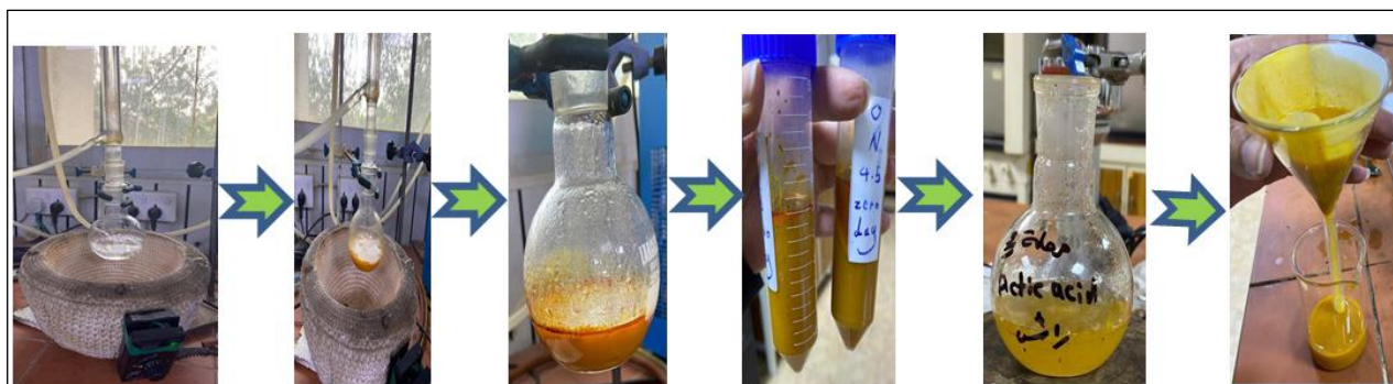
Figure 2: A Ex/Chitosan nanoencapsulation biosynthesis process.
