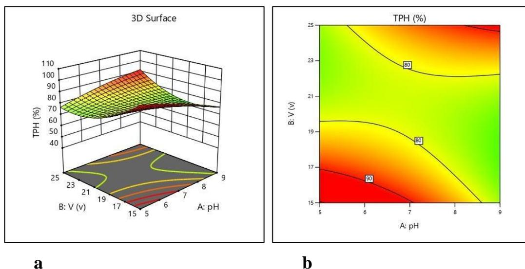
**Figure (4):** (a) 3D drawing and (b) a layered drawing showing the relationship between pH and voltage in removing total petroleum hydrocarbons from laboratory polluted water using aluminum plates.
