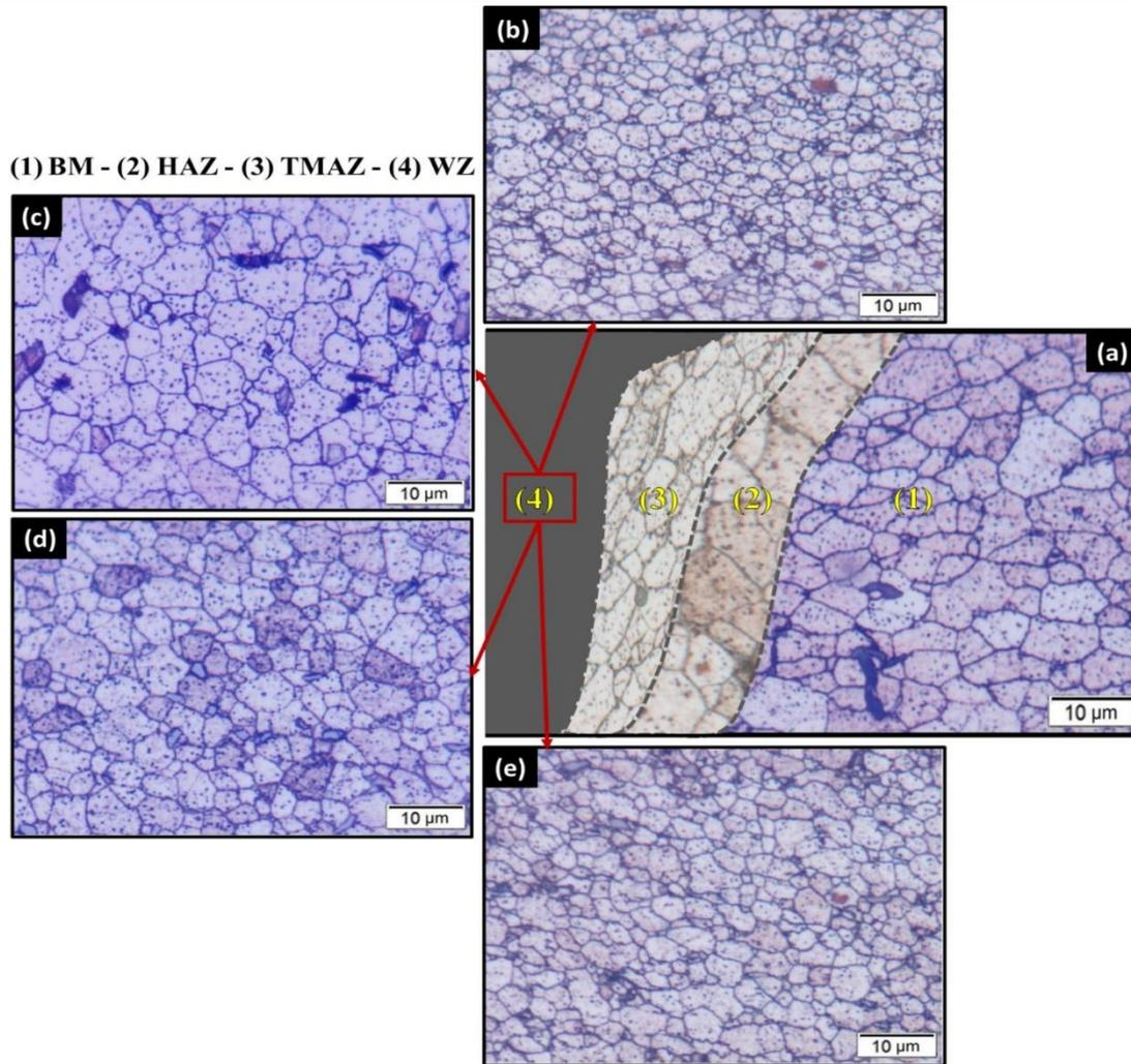
**Figure 9:** Microstructures in the AA6082 FSWed joints of (a)BM, HAZ, and TMAZ regions. The microstructure and composition of the nugget region for (b) E0, (c) A0, (d) E3, and (e) A3 joints.
