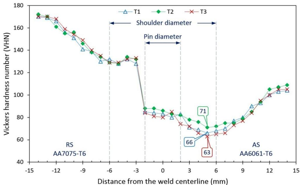
**Figure 11.** The distribution of hardness around the perimeter of the weld is dependent on the design of the pin.
