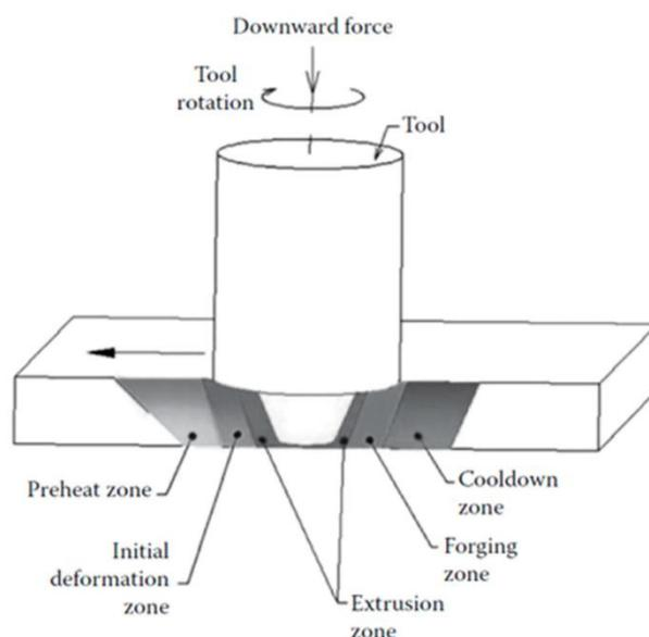
**Figure 1. Stages in the Friction Stir Welding (FSW) process**
