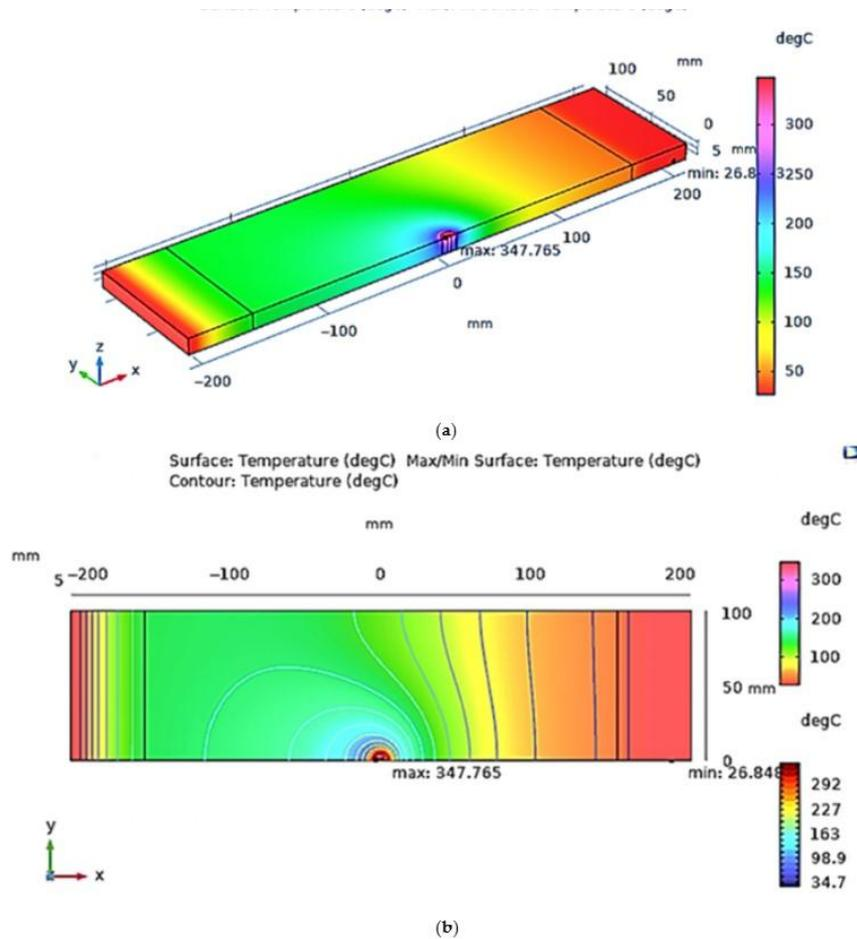
**Figure 8.** (a) Temperature distribution on the Al 6061 T6 plate and (b) temperature contours on The Al 601 T6 plate
