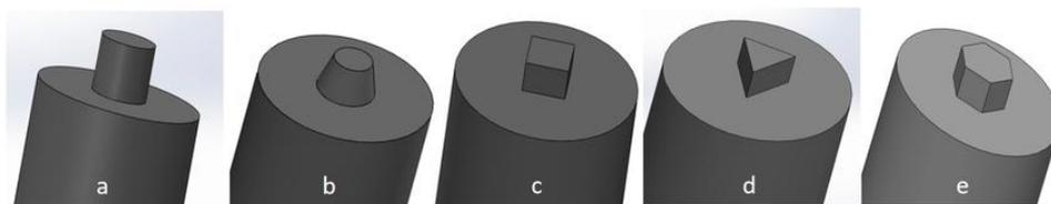
**Figure 3. FSW tools with different pin profile (a) cylindrical; (b) tapered cylindrical; (c) triangular; (d) square and (e) hexagonal.**
