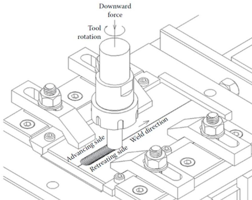
**Figure 2. Schematic of FSW process**
