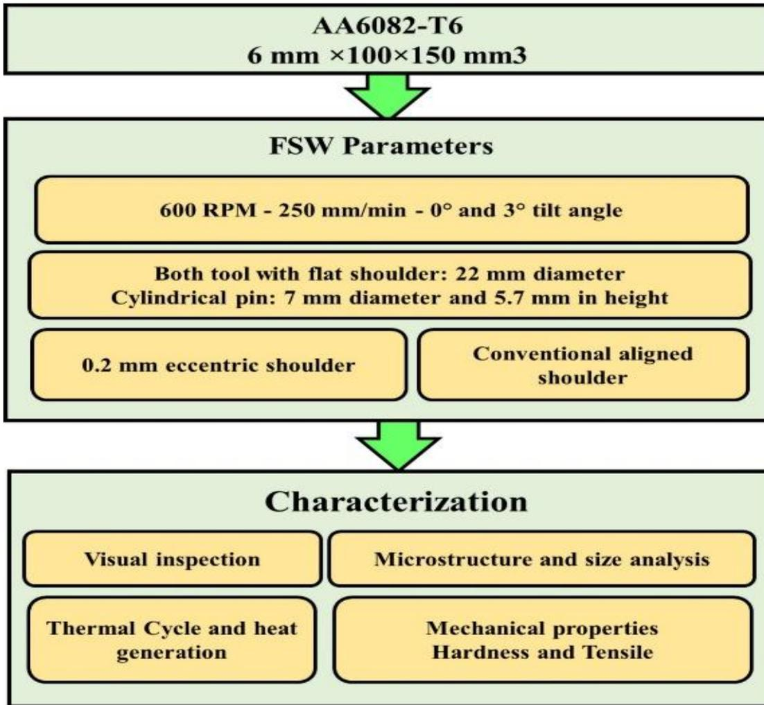
Figure 4. Experimental procedure flowchart of the applied FSW of 6
