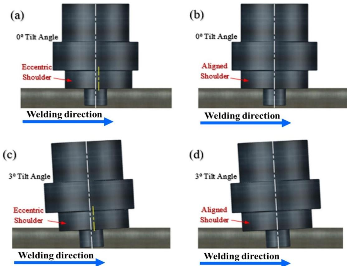
**Figure 7.** Schematic of the FSW processes involved: (a) eccentric shoulder, 0°tilt angle, (b) aligned shoulder, 0°tilt angle, (c) eccentric shoulder, 3°tilt angle, (d) aligned shoulder, and 3°tilt angle.
