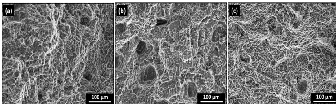
**Figure 10.** Fracture surfaces of the tensile tested specimens of (a) AA6082-T6 initial plate and FSWed joint s of (b) E3, and (c) E0.
