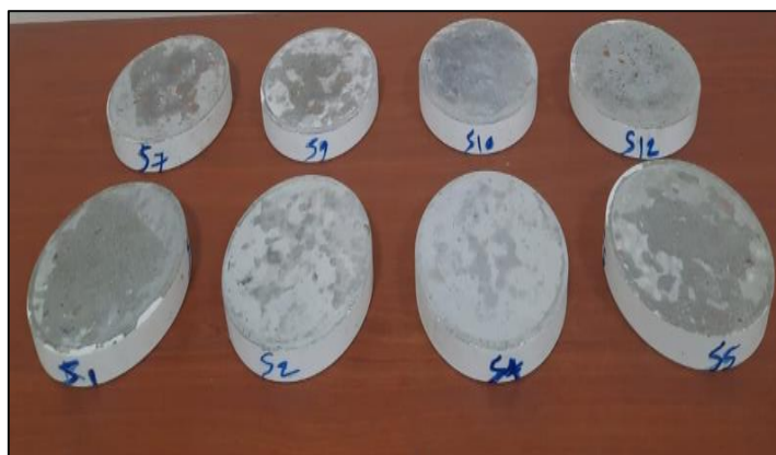
Fig. 5. Shows specimens for the thermal conductivity test.
