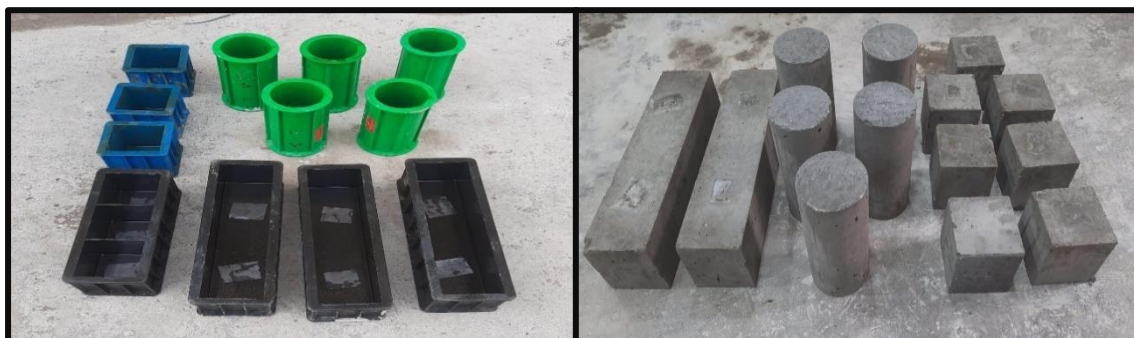
Fig. 2. Shows preparation of molds and castings.
