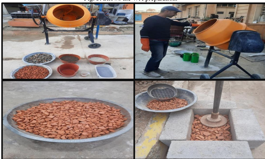
Fig. 4. Shows the preparation of OPC, WA and CCB.
