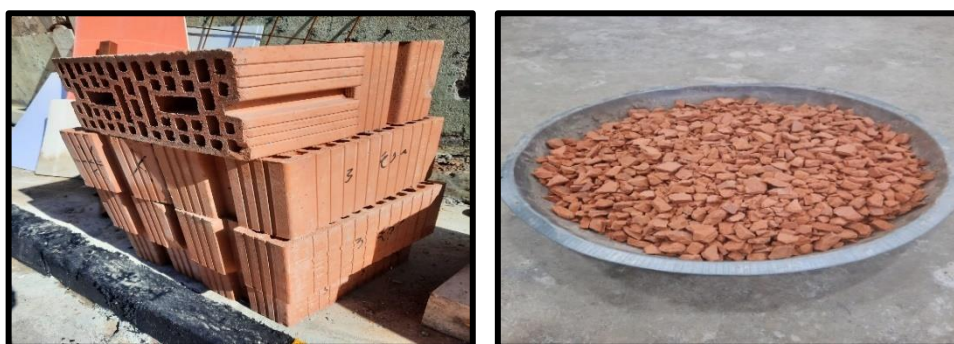
Fig. 1. (b) Shows Crushed Clay Blocks.
