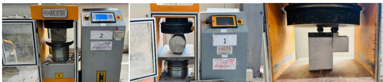
Fig. (3): Compressive strength test, splitting tensile strength test, and shear strength test.
