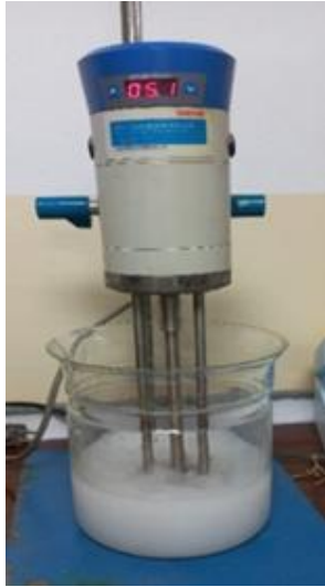
Fig. 2. Preparation of the oil-in-water emulsion using the high-shear emulsifier device.
