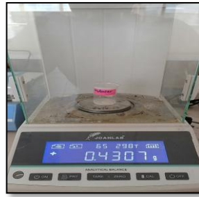
Figure (3): A digital balance for weighing the specimens for water sorption and solubility.
