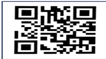
Figure (4) shows the shape of version 2, size 25×25, quantity 20-47, character/digital code.
