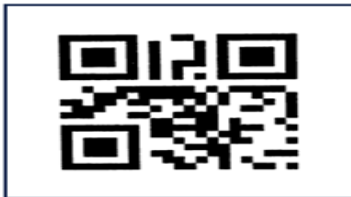
Figure (3) shows the shape of version 1, size 21×21, quantity 10-15, character/digital code.
