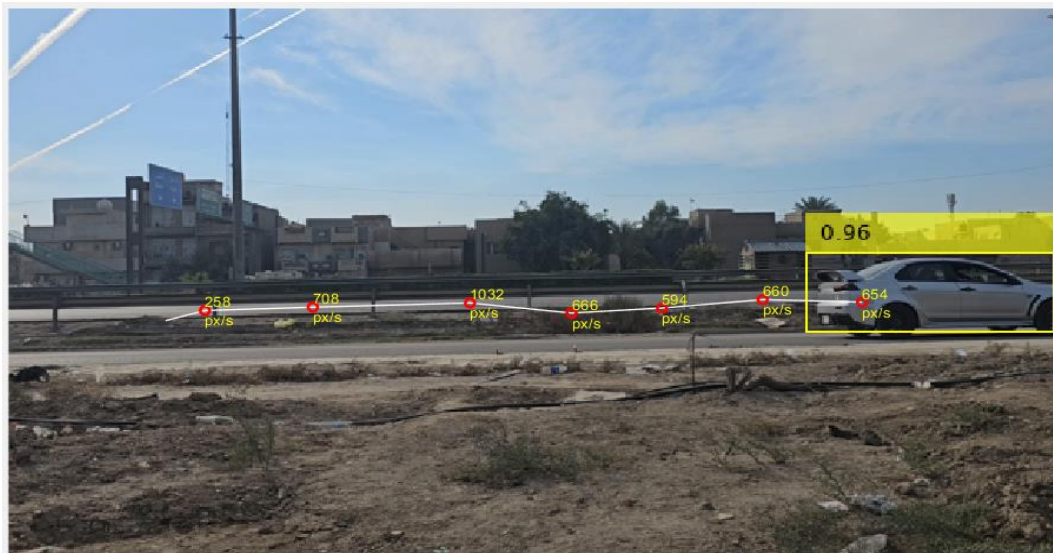
Fig.2. Shows the approximately linear path of the vehicle and specifies the speed in pixel/sec.
