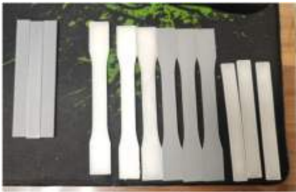
Fig. 2. Tensile and bending specimens fabricated using FDM.
