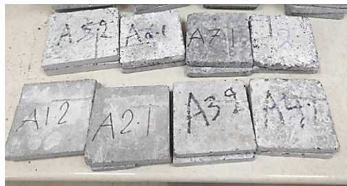
Fig. 5. Thermal Conductivity samples
