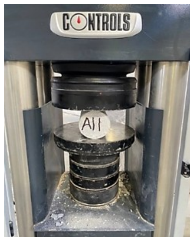
Fig. 3. Splitting tensile strength machine
