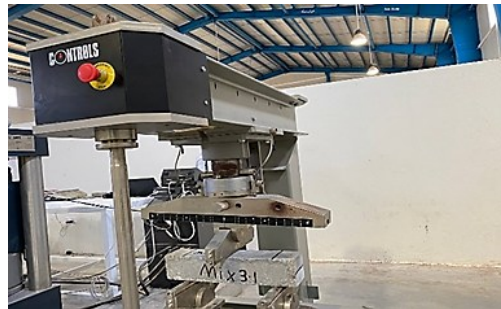
Fig. 4. Modulus of rupture machine
