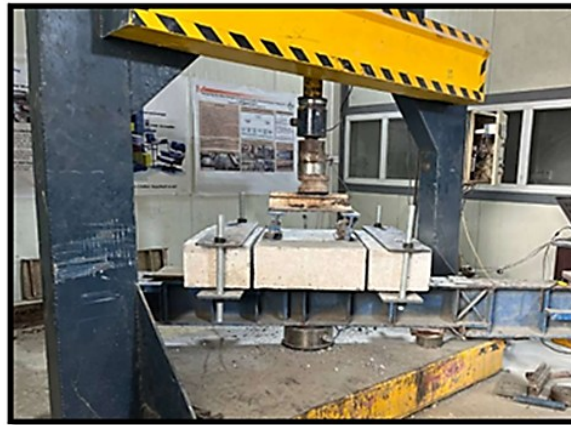
Fig. 6. The testing machine with the specimen
