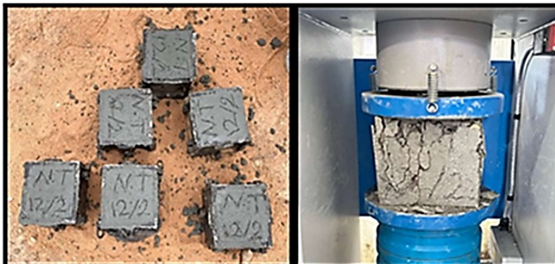
Fig. 5. Casting and testing cubes
