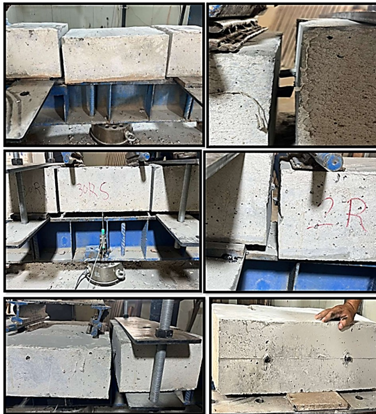
Fig. 8. GFRP dowel bar failure
