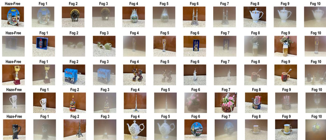
Fig. 5. Real haze generation taken with a household steam iron, showing real-world fog applied to indoor scenes. A total of 616 images were created across ten fog levels for increased realism beyond synthetic evaluations.
