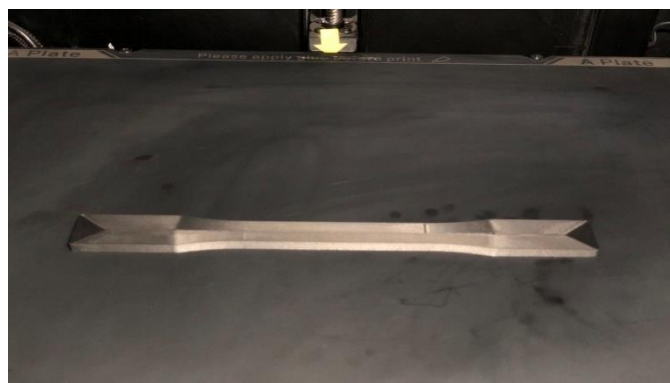
Figure 7. Tensile Test Specimen
