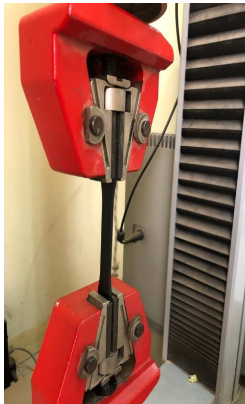
Figure9. Tensile Test Device
