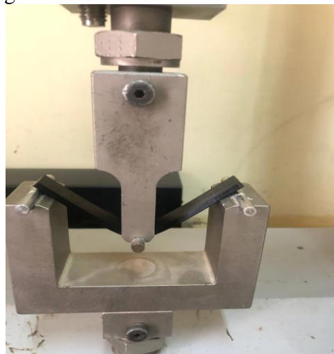
Figure12. Flexural Bend Testing Specimen
