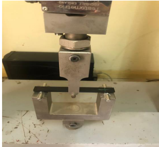
Figure11. Bending test Device
