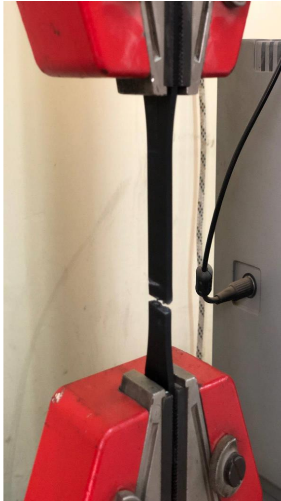
Figure10. Tensile Testing Specimen
