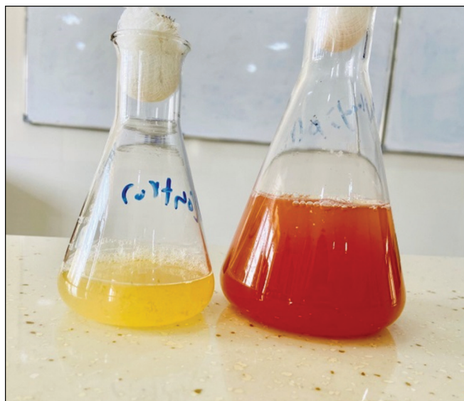
Figure 2: Visual observation of iron oxide NPs formation by color changing from light yellow to red after 48 h
