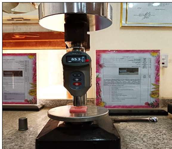
Figure 2. Surface hardness testing by Shore D durometer
