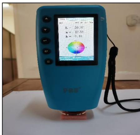
Figure 3. Color change test by colorimeter
