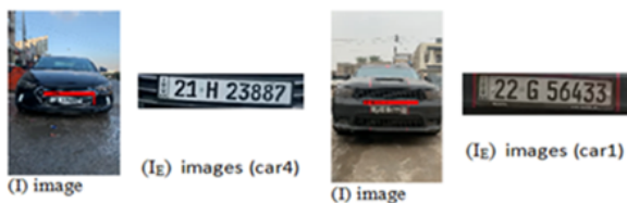
Fig. 8 Extract the plate region from the image using RCNN-det model to create DB2.
