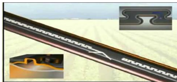
Figure (1) Ro-Drip-Drip Tape subsurface drip irrigation pipes. The figure shows the drippers that discharge irrigation water.
